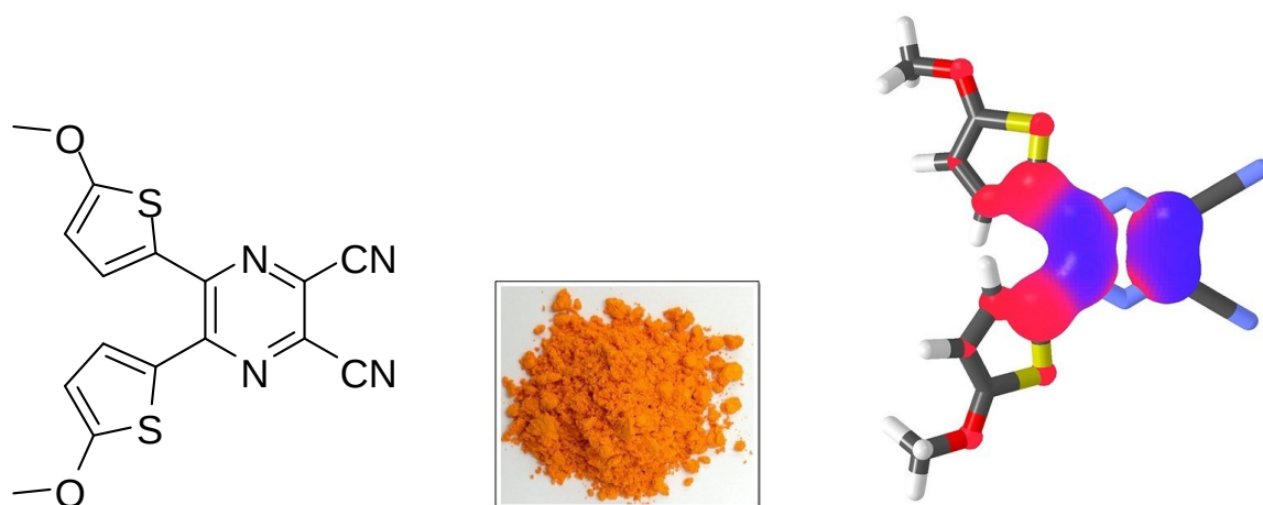
Figure 1: structure of DPZ catalyst, bulk, and HOMO/LUMO localization.
